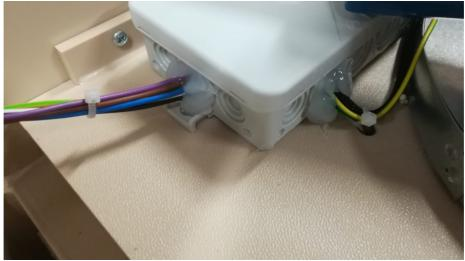
In addition, check the cable entry from the tank to the incubator for leaks, seal with silicone if necessary.
