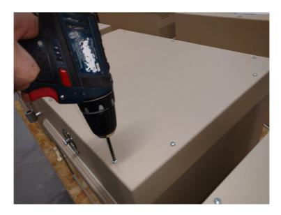
**step 3:** Remove the old fan hood, unscrew the 4 screws and remove the cabels in the terminal box with a suitable screwdriver. Then take the hood upwards.
