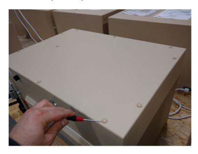
**step 2:** Unscrew the screws and remove the cover (if necessary use a bit more force, the cover is partially glued).
