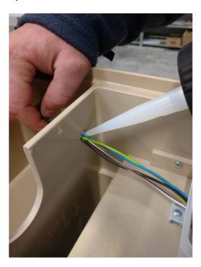
**step 6:** Mount the lid of the terminal box. The edge, which is marked red in the following picture, has to be glued with silicon.
